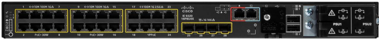
Figure 7. IE-9320-16P8U4X Switch with multi-gigabit and 4PPoE
