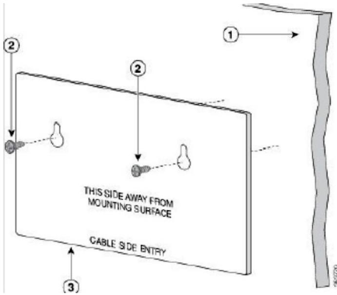
**Step 7** Remove the screw template from the wall.
