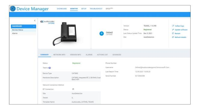
Network administrators can get logs from devices for debugging purposes without needing to go to the device The Collect Logs option in AudioCodes' Device Manager, shown in the next figure, allows this. Network administrators can navigate to the option via Monitor > Dashboard > Devices Status and then click Actions = next to the device.
