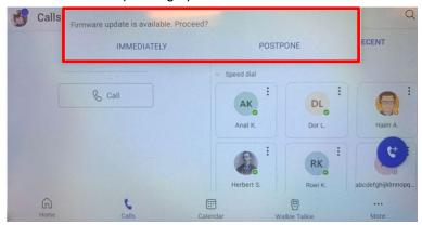
When any update is pushed to the device, the device's firmware detects whether the user is actively using the device. After determining this, an appropriate message and options are provided for the user to either delay the update or apply it immediately.
