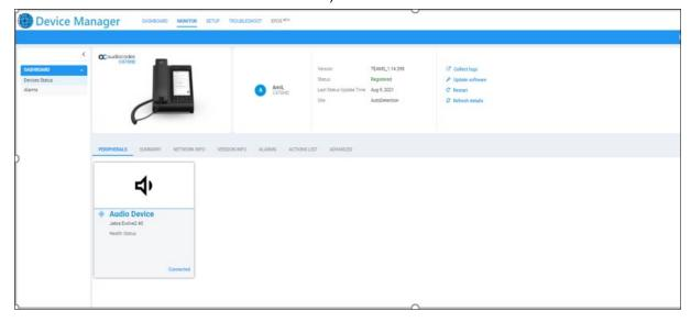
The Show Info screen displays all information related to the device needed by the network administrator. The **Peripherals** tab is displayed (by default) if a peripheral such as a headset is connected, as shown in the previous figure. All information that the peripheral device sends to the OVOC as raw data composes the Peripherals screen.
