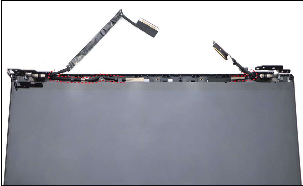
Figure 1-35. Unrouting the Cables
