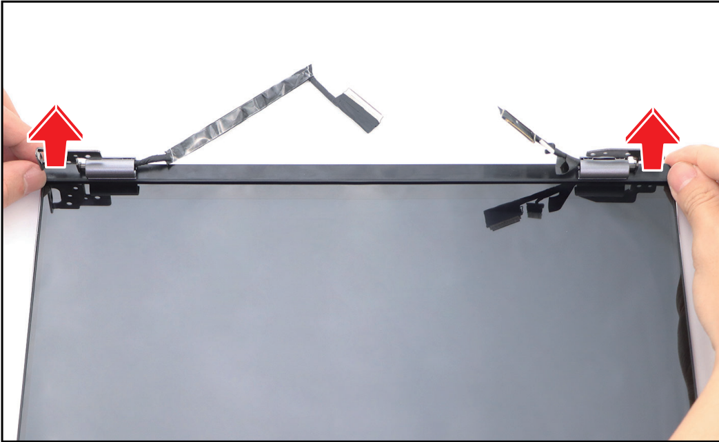
Figure 1-33. Removing the Strip Bezel
