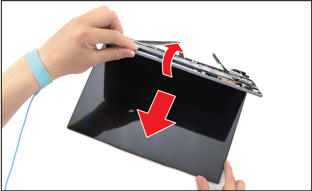
Figure 1-27. Removing the LCD Module
