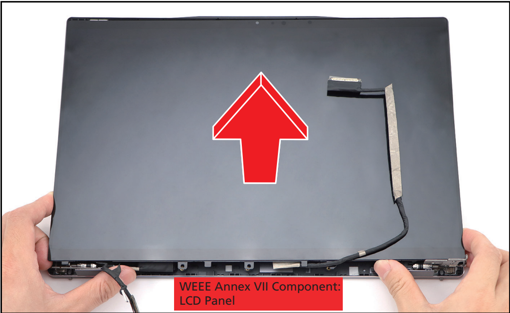
Figure 1-38. Remove the LCD Panel
