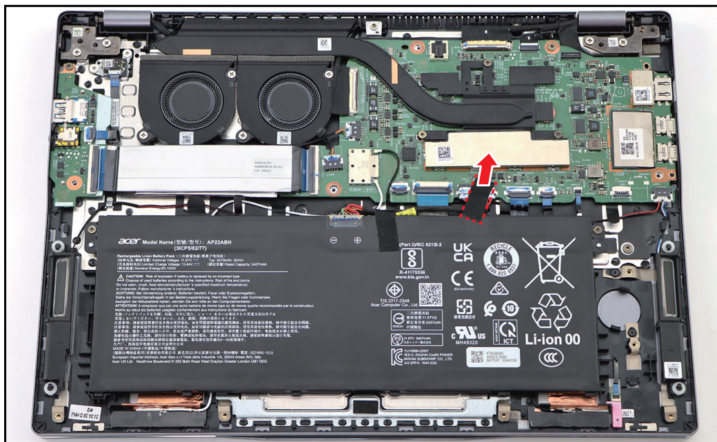
Figure 1-5. Detaching the Acetate Tape
