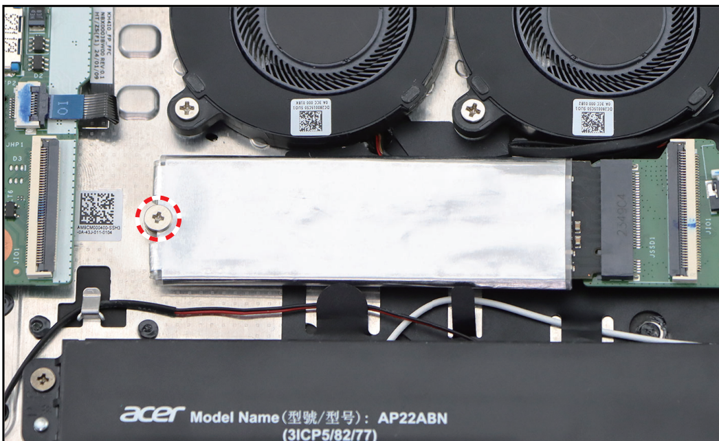
Figure 1-11. Removing the Screw
