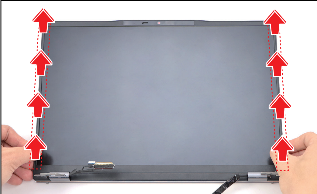
Figure 1-41. Removing the LCD Bezel (2 of 3)
