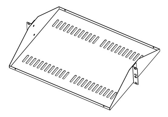
2U Universal Cantilever 14in (350mm) Vented Center Rack Shelf for 2-Post Rack
