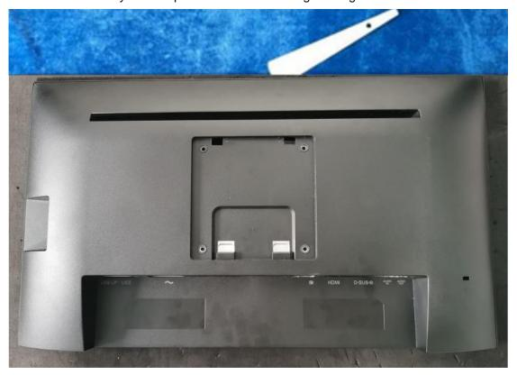
4. Remove the rear cover, then take off all of the tapes and disconnect the connectors.
