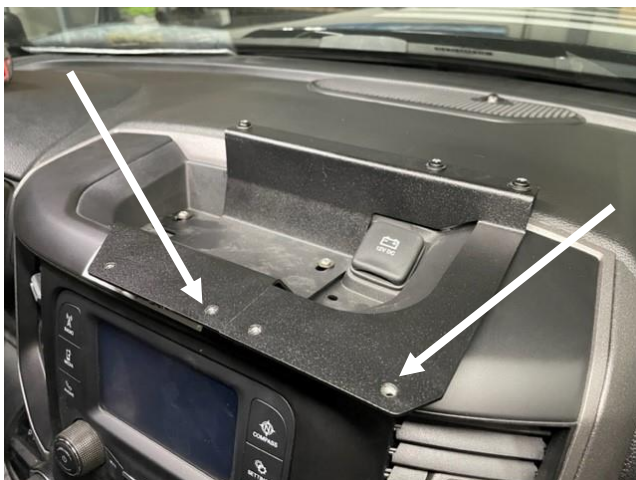
Attach main frame / hinge assembly to top tray / bracket with (4) 10/32 x 1/2 screws and flat washers.
