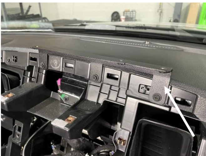
Attach upper mount bracket (27146) to dash using previously removed OEM screws.
