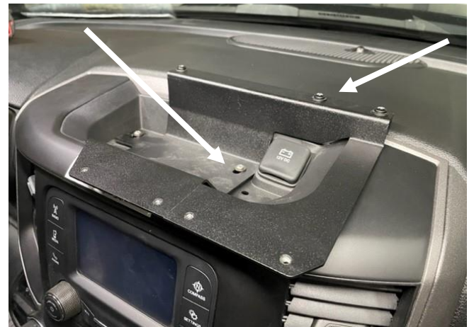
Attach top tray / bracket (27147) to Upper bracket with (3) 10/32 x 1/2 screws and flat washers. Also attach tray to dash with (2) 8 x 1-1/2 PPHSMS and flat washers.
