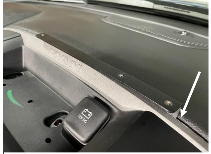
Reinstall center instrument panel. Upper bracket will come out through the small gap in trim panel.
