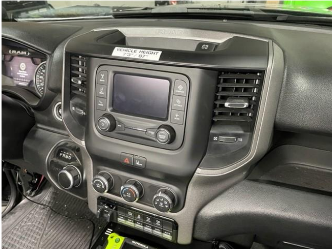
Dodge Ram Pickup dash with Uconnect® 3 Radio with 5-Inch Display prior to installation.
