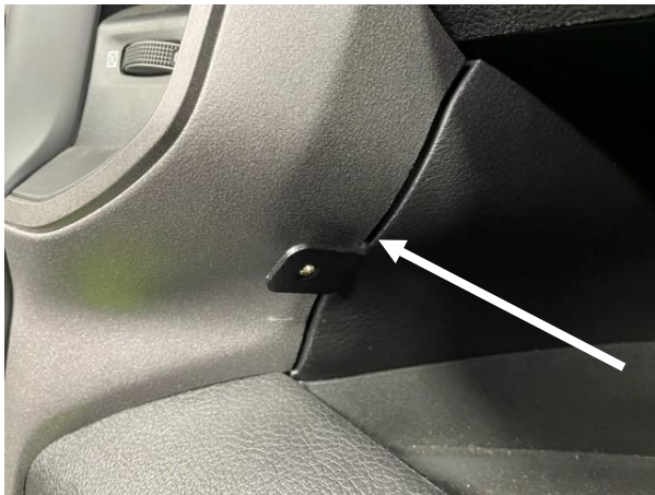
Reinstall center instrument panel. Lower bracket will come out through the small gap in trim panel.
