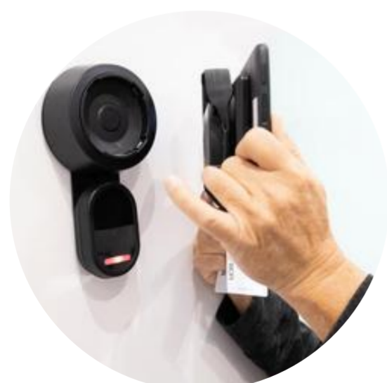
One-handed dock and undock with magnets and latches.
