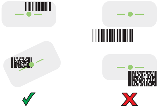
Figure 14 RS6100 Aiming Pattern
