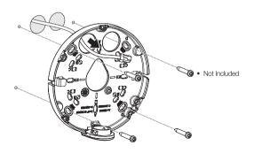
Installing using pipe
