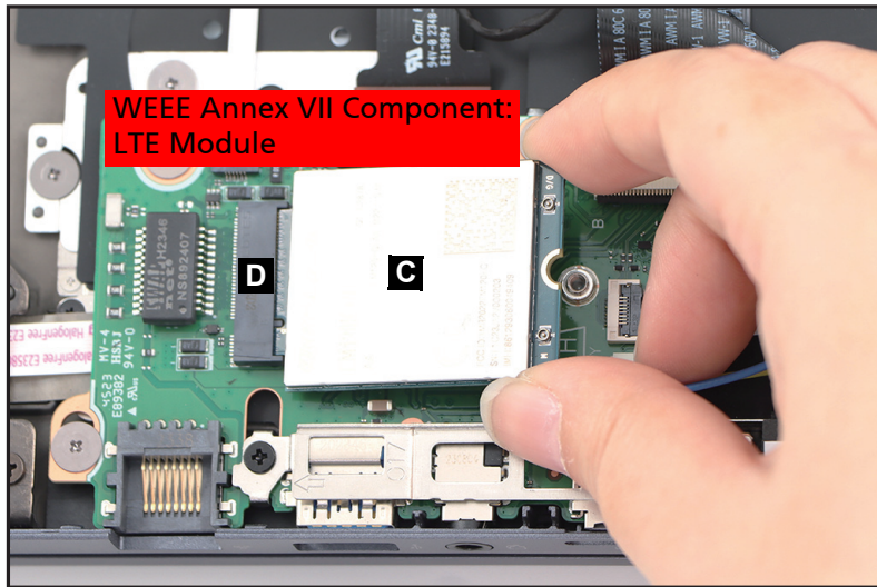
Figure 1-21. LTE Module Removal
