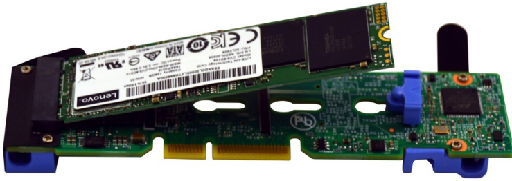
Figure 3. Dual M.2 Adapter and a 128 GB M.2 drive
