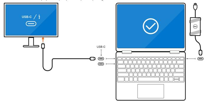
• Connect an external display using a USB-C to Thunderbolt/HDMI/DisplayPort adapter:
