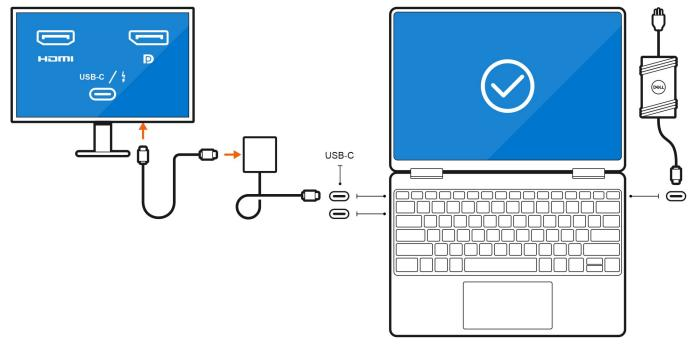
• Connect up to three external displays using a USB-C docking station or USB-C to Thunderbolt/HDMI/DisplayPort adapter:
