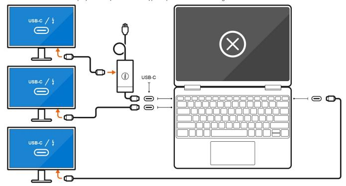
• Connect up to four external displays directly to the WD19TB series docking station and than connecting the docking station to the computer:
