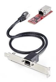
This 2.5 GbE M.2 Network Interface Card (NIC) features an Intel I225-V chipset with Intel vPro technology, for enhanced performance and data integrity. Variable multispeed options (2.5/1Gbps and 100/10Mbps) enable support of new and legacy network hardware. Leverage existing Cat5e or CAT6 cabling infrastructure while adding 2.5GBASE-T (802.3bz) compatibility for seamless integration.
