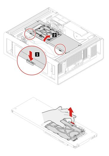
Disconnect the cable from the hard disk drive after detaching the storage drive bracket from the optional hard disk drive bracket. Then, remove the bracket.
