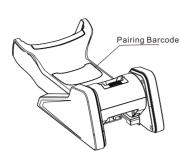
The scanner and the cradle are paired before shipping. Before pairing other scanners, disconnect or power off the paired scanner and scan the pairing barcode in the cradle
