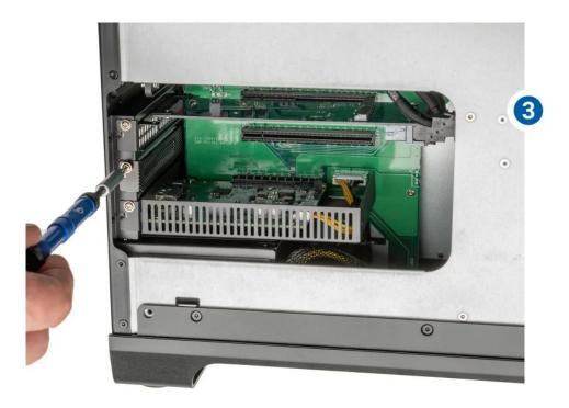
**4.** Align your PCIe card's connector with the open slot then install the card as you normally would when installing into a desktop computer.
