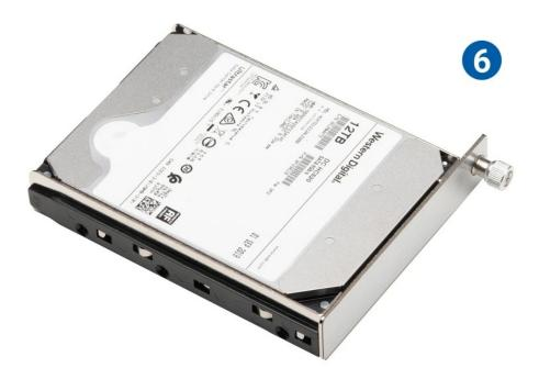
7. Fasten the drive into the drive tray using six of the included screws (three per side).
