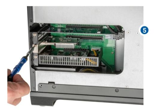
**6.** If your PCIe card has I/O Ports, double-check the back of the device to ensure the bracket is level / that none of the ports are obscured by the plating on the back of the case. If needed, loosen the screw you set in Step 5, re-align bracket as needed, and re-tighten the screw.
