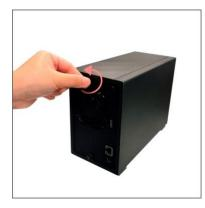
2. Place the device sideways on a flat surface. Note the wording indicating the directions for opening and closing the cover. Remove the cover by sliding it in the direction shown in the graphic below.
