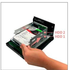
Note: Please insert the hard disk into the HDD 1 slot shown in the graphic in order to have it initialized.
