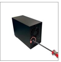
4. Position the bracket over the hole for the removed fan screw. Secure the bracket in place by replacing the fan screw.
