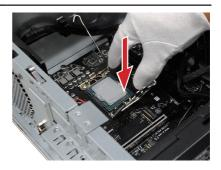
5. Close the load plate, and then close the load lever. Evenly spread a thin layer of thermal paste on the top of the CPU. This will help in heat dissipation and prevent CPU from overheating.
