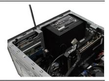
9. Connect the power cable and signal cable.
