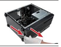
2. Unlock the screws on the rear side, and keep the screws for later use.
