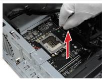
3. Next, open the load plate fully and carefully.
