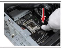
2. Open the load lever fully and carefully.
