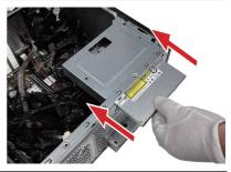
3. Lock the screw to secure the ODD.
