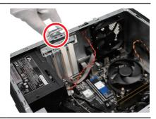
2. Locate the VGA card slot. Keep the gold fingers and the slot aligned, and push the VGA card till it can not go futher.
