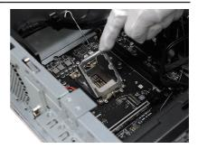
4. Align the notches with the socket alignment keys. Lower the CPU straight down, without tilting or sliding the CPU in the socket. Inspect the CPU to check if it is properly seated in the socket.
