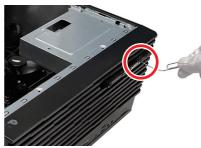
7. Align the hooks on the front bezel with the holes on the ODD and install it carefully.
