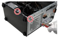
3. Locate the 1 screw between HDD tray and power suppy. Unlock it on the chasis, and keep it for later use.
