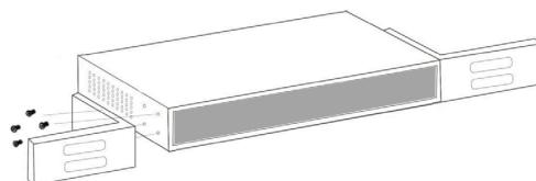
Use the screws provided with the equipment rack to mount the Intellinet Network Solutions data switch on the rack.
