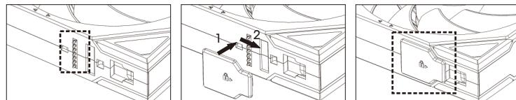
**!** Exposed POGO PIN terminals can easily short-circuit metal components if touched accidentally. It is recommended to cover with pin cover for protection/POGO PIN端子外露容易誤觸金屬造成短路,建議裝上塑膠薄片保護/
