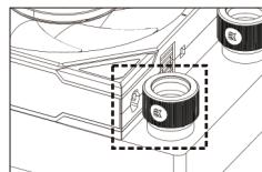
**Note!** If the radiator outlet affects the fan interlocking key, you can remove them/若遇到水冷
