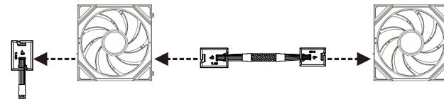
**!** Connect to UNI FAN TL Series Controller(Each port supports a maximum of 10 TL fans, while the controller supports a maximum of 16 fans in total)/
