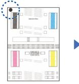
Follow the LCD instructions to print the Adjustment Sheet. The black circle mark is located in the upper left corner of the sheet.
