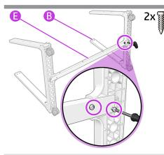
Fix the bottom cross tube (E) to the right bottom connector (B) with two T25 screws.
