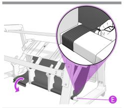
Attach the basket to the bottom cross-tube (E) using the Velcro strap.
