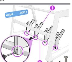
Fix the four stacker support-adaptors (I) onto the bottom cross-tube (E) using four T25 screws.
