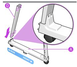
Insert the right rear-leg (D) onto the rear of the right-bottom cross-connector (A).
