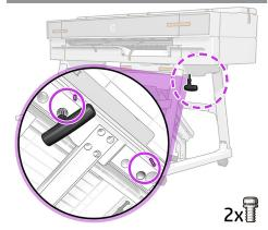
From underneath, fix the right side of the printer to the stand with two T25 screws.
