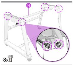
Fix the top cross-beam (H) to the stand using four T25 screws on the left and right side.
