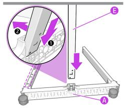
Important: The holes must face inwards. Insert the bottom cross-tube (E) diagonally into the left bottom-connector (A) and push it into place.
