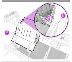
Important: Make sure that the sheet organizer (M) also fits onto the stacker adaptor pin as shown (K). Remove the packaging from inside of the sheet organizer(M).
