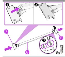
Insert diagonally the left and right brackets (F) into the rear cross-tube (G).
