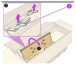
Remove the four Stacker support Adaptors (I) on the top of the stacker.
