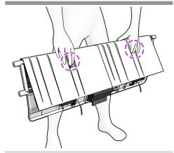
Important: Use the square finger grooves on the stacker to hold it. The black pin should be facing downward.
