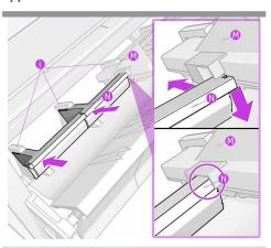
Pull down the stacker tray and slot the side blocker (N) into the unused stacker support-adaptors (I) at the left. Pull up the sheet organizer (M) until it aligns and fits with the side blocker (N), then remove the orange tape.
