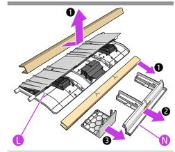
Remove the cardboard from the stacker tray (L). Remove the side blocker ( $\mathbb{N}$ ) and the cable cover.
