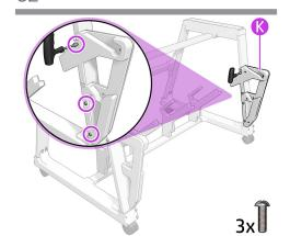
Fix the right stacker-adaptor (K) onto the front right-leg with three T25 screws.
