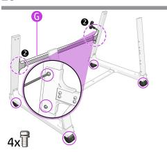
Rotate the assembled stand and place it on the table with the wheels facing down.
