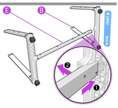
Insert the bottom cross tube (E) diagonally into the right bottom connector (B).
