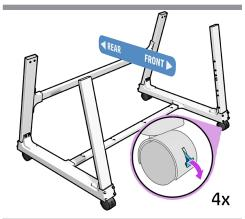
Place the stand upright and check the four wheels are locked.
