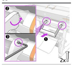
Install the U-frame  $(\bigcirc)$  onto the front of the printer and fix it in place using two T20 screws.
