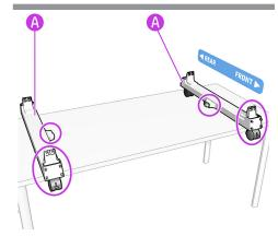
HP recommends completing the assembly on a table. Remove the two bottom cross-connectors (A and A) from the box.
