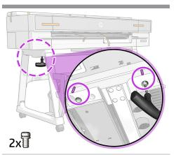
From underneath, fix the left side of the printer to the stand with two T25 screws.
