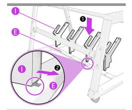
Position the four stacker support-adaptors (I) on the bottom cross-tube (E); insert and rotate, then slide and push to install them one-by-one.
