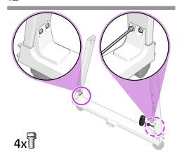
Fix the legs in place with two T25 screws each
