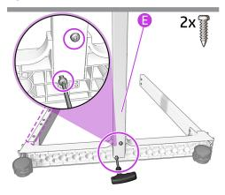
Important: The holes must face inwards. Fix the bottom cross-tube (E) to the left foot using two T25 screws.
