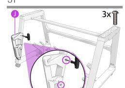
Fix the left stacker-adaptor (J) onto the front left-leg with three T25 screws.
