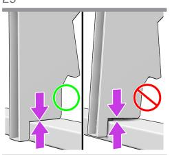
Make sure the four stacker support-adaptors (I) are correctly installed.
