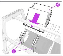
Remove the Sheet Organizer (M) from the bag and slot the two stacker suppport adaptors (I) at the right.
