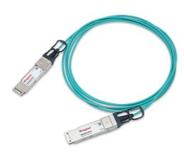
4m Mellanox/NVIDIA MFA1A00-C004 Compatible 100GBase-A0C QSFP28 to QSFP28 (MMF, 850nm, LSZH) Active Optical Cable
