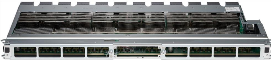
Figure 16. Cisco Nexus 9800 fabric module
