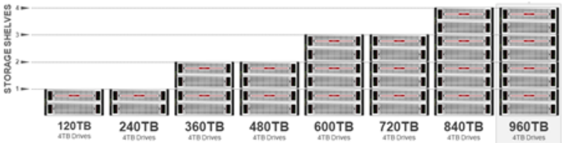
Figure 2-1 5U84 Storage Shelf (capacity with 4TB drives (half and full))
