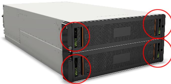
Figure 2-10 Drawer Sideplane Status panel locations
