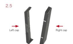
On the front of the storage shelf, reattach the left and the right caps. The left cap contains the control panel. The right cap contains spaces for two latches which connect to the storage shelf.
