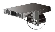
Secure the captive screws onto the node ears.
