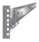
Place one rail inside the rack. Use the same 1 RU space and holes in the front and rear of the rack. Align the pins in the top and bottom holes of the top RU. Move the front and back of the rail to fit into the rack. Slide the rail forward until the pins click into the rack holes
