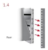
Extend the rail assembly to enable the rear rail pins to engage. Verify that the pins are fully seated in the holes in the rack posts. Secure the four adjuster screws as needed.
