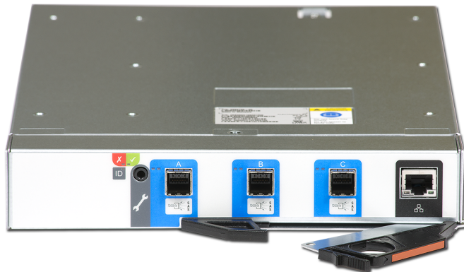
Figure 2-6 Veritas U12 65.5TiB/72TB Storage Shelf I/O module
