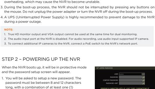
To prevent the NVR from overheating, do not operate it in an area that exceeds the maximum recommended ambient temperature of 104°F (40°C). To prevent airflow restriction, allow at least
