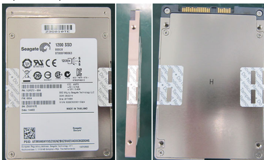
Figure 7 Example of FIPS tamper evidence labels
