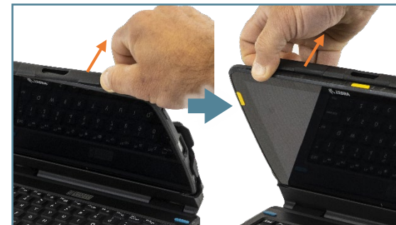
On both sides, push up on Top Latch Ridge & pull forward on back corner of Tablet
