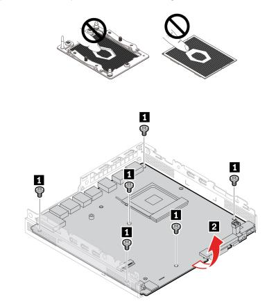
**Note:** The failing system board must be returned with a microprocessor socket cover to protect the pins during shipping and handling.
