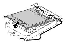
3. Carefully check the four corners of the socket cover to ensure that the cover is seated securely.
