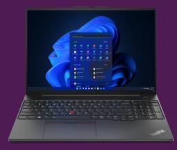
The 16" screen has an optional multi-touch functionality that lets users naturally interact with the device and an anti-glare surface that makes it easier to comfortably work in bright-light conditions. The 16:10 aspect ratio and 100% sRGB color gamut present stunning and true-to-life visuals.
