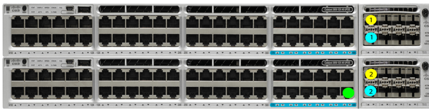
Dual 10/25GE ToR Switches (standalone or stacked)
