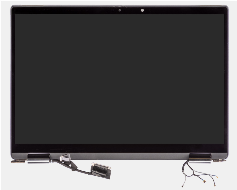
Figure 1. Display assembly without WWAN-antenna cables
