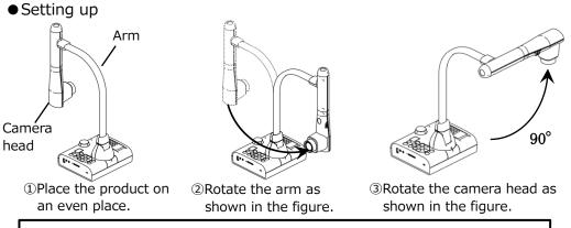
Caution Hold the arm when rotating the arm. Do not hold the camera head.
