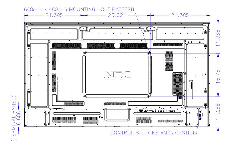
NEC strongly recommends using size M8 screws (16 - 18mm + the thickness of the bracket and washers in length).
