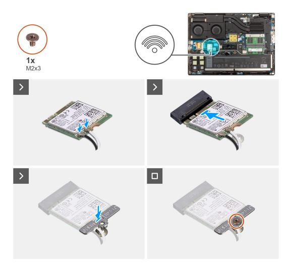
1. Connect the antenna cables to the WLAN card.
