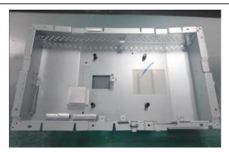
Take out the Thermal pads from Power PCB
