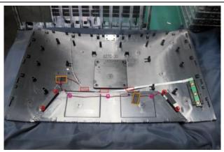
Remove 1pcs aluminum foil, 2pcs acetate tape and 1pcs conductive tape.
