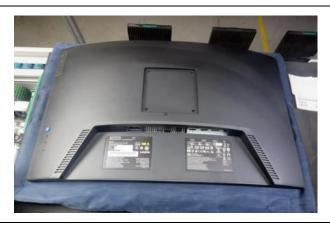
Wedge your fingers between the rear cover and the middle bezel on the corners of the top side of the monitor to release the rear cover.
