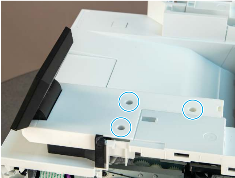
Figure 4-765 Remove three screws
