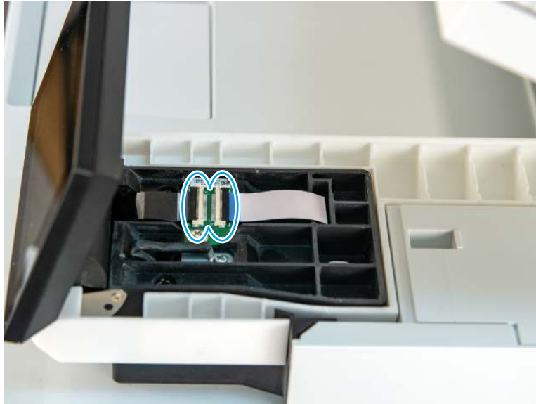
Figure 4-41 Disconnect two FFCs
