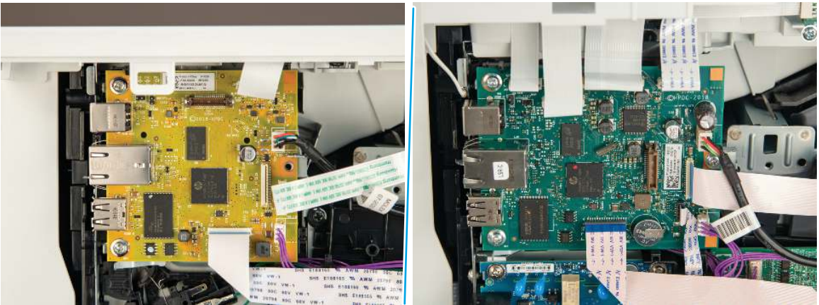
Figure 4-716 Disconnect all of the connectors (SFP/MFP)
