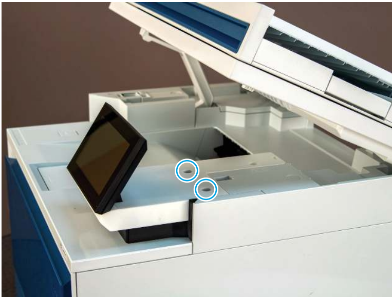
Figure 4-39 Remove two screws
