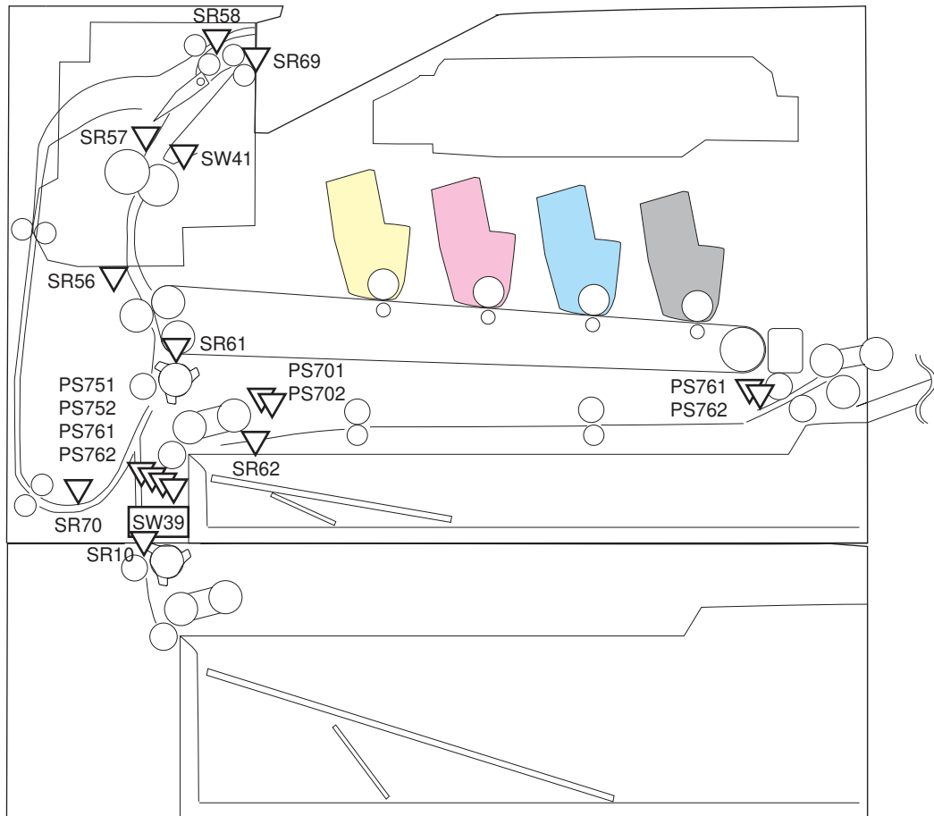
Figure 3-6 Sensors and switches (base printer)
