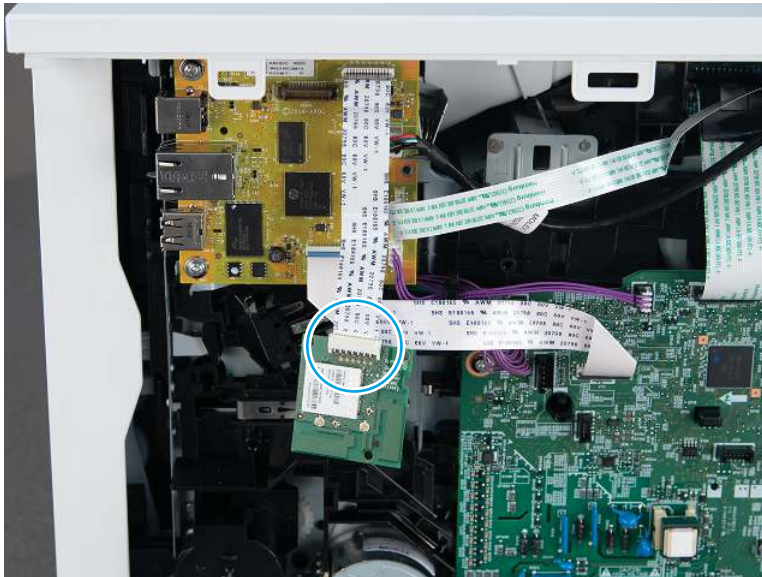
Figure 4-251 Remove the PCA
