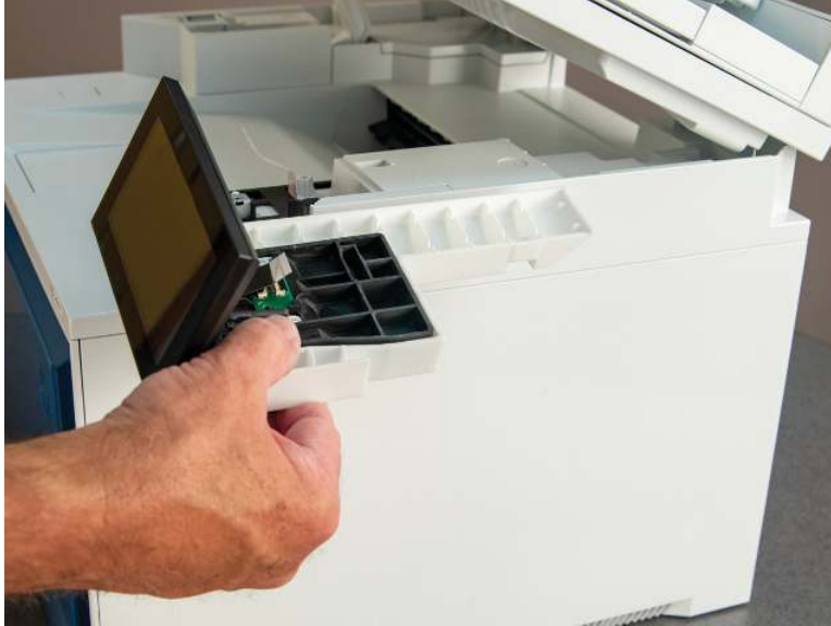
Figure 4-44 Remove control panel and mount base
