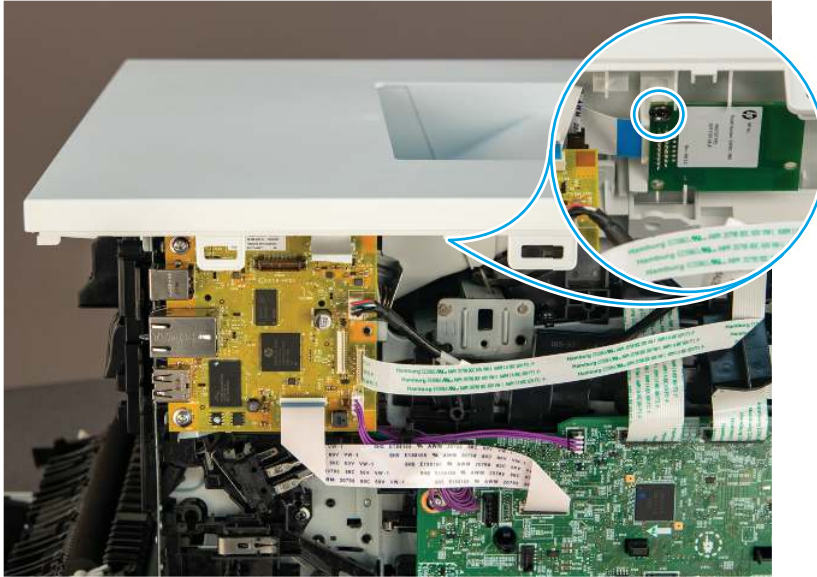
Figure 4-389 Remove one screw
