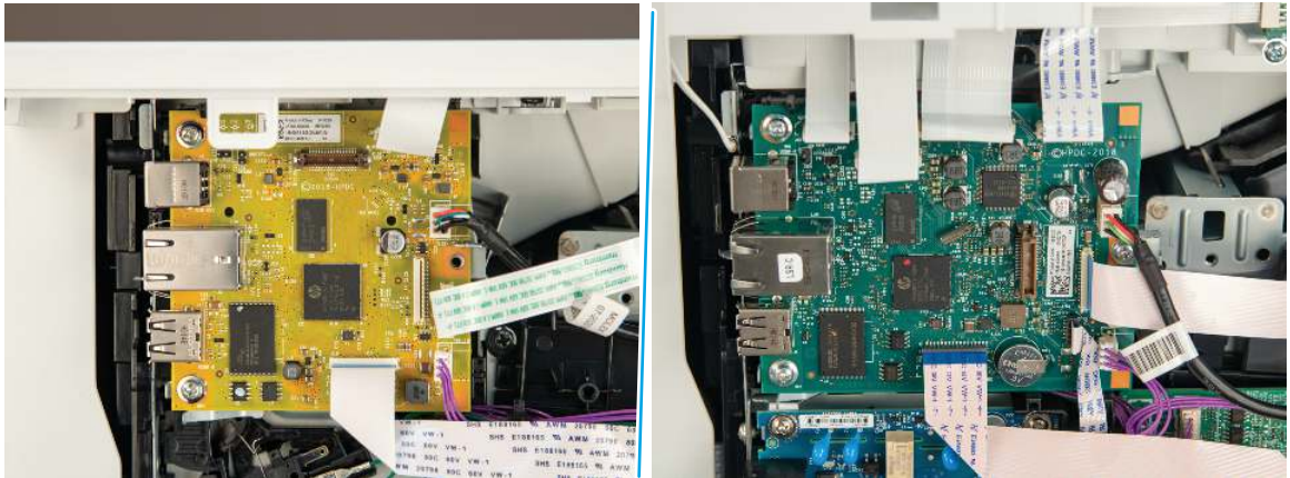
Figure 4-656 Disconnect all of the connectors (SFP/MFP)
