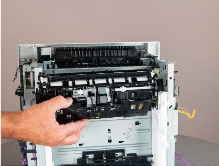
Figure 4-1069 Remove the feed upper guide assembly
