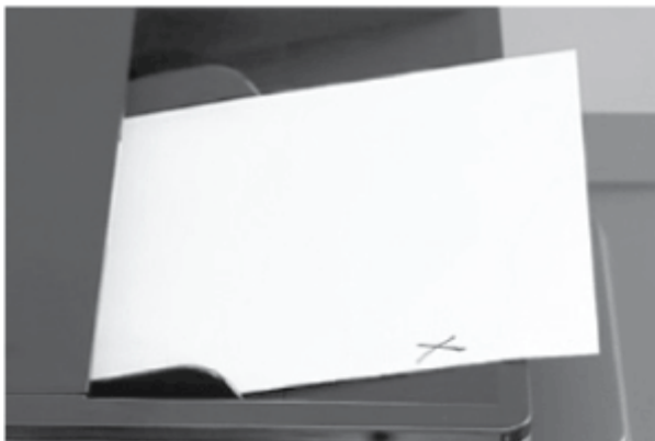
Figure 3-37 Load the document feeder
