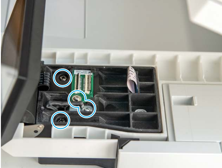
Figure 4-42 Remove four screws
