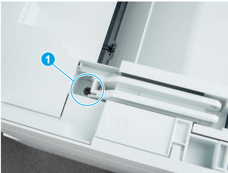
Figure 4-10 Remove one screw
