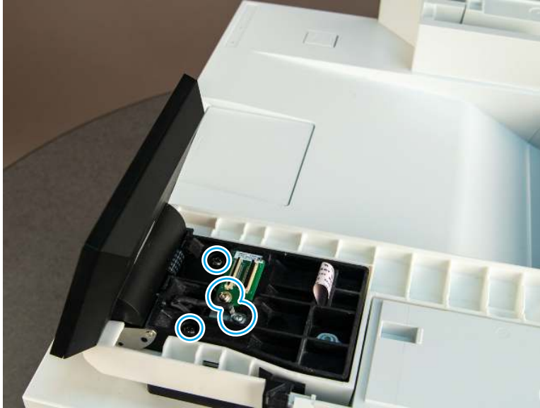
Figure 4-235 Remove four screws
