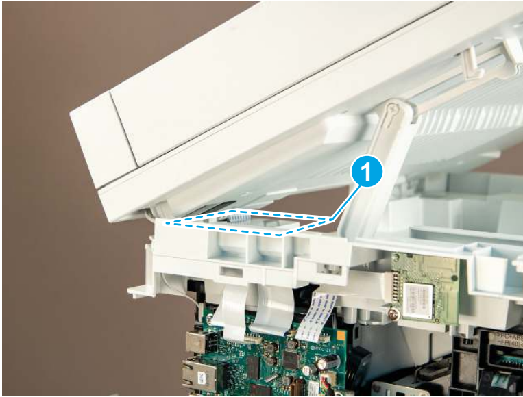
Figure 4-370 Remove the FFC cover
