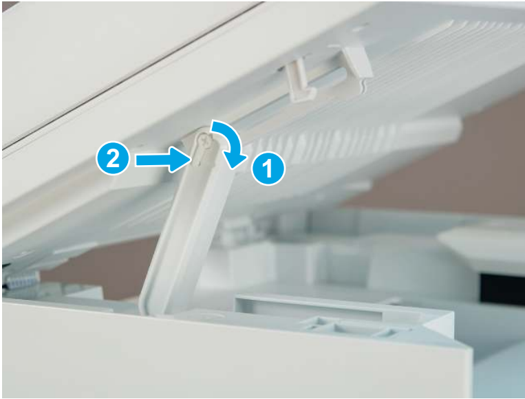
Figure 4-38 Reinstall the slider pin
