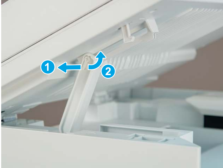
Figure 4-36 Remove the slider pin
