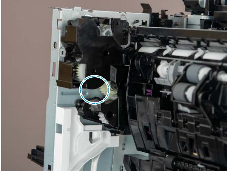
Figure 4-1127 Release one tab
