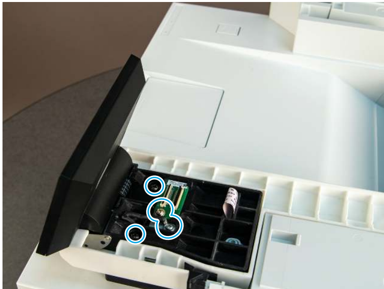
Figure 4-164 Remove four screws
