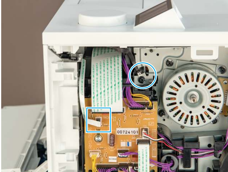
Figure 4-507 Disconnect one FFC and remove one screw
