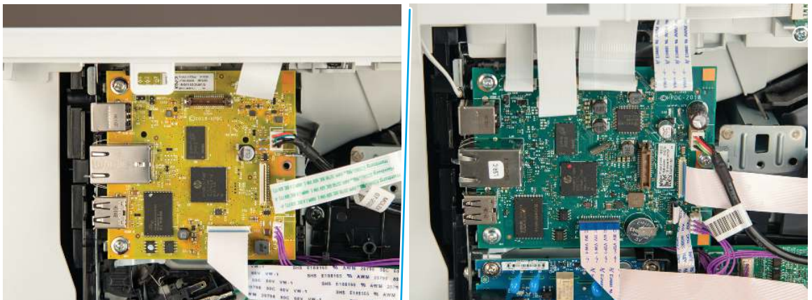
Figure 4-844 Disconnect all of the connectors (SFP/MFP)
