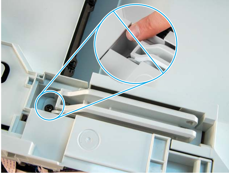
Figure 4-157 Remove one screw
