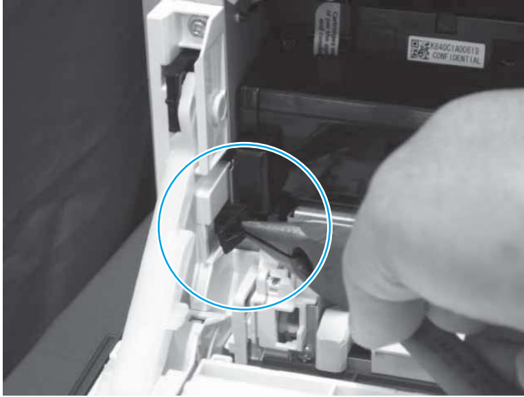
Figure 4-823 Remove the stopper (left side)
