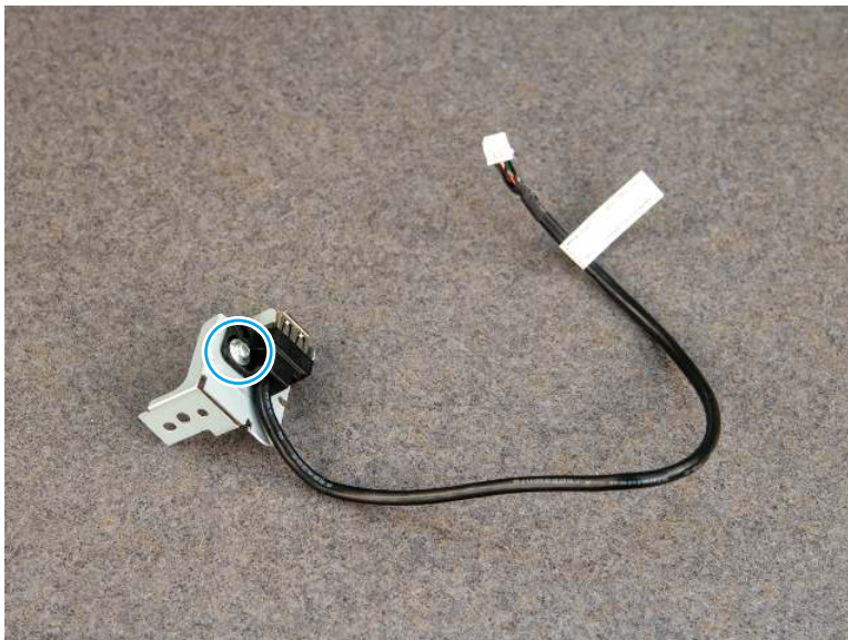
Figure 4-241 Separate the assembly from the bracket
