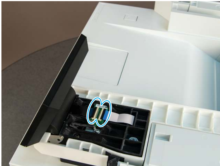
Figure 4-400 Disconnect two FFCs
