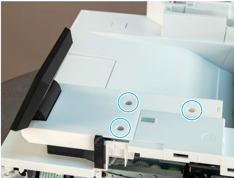
Figure 4-603 Remove three screws
