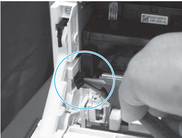
Figure 4-437 Remove the stopper (left side)
