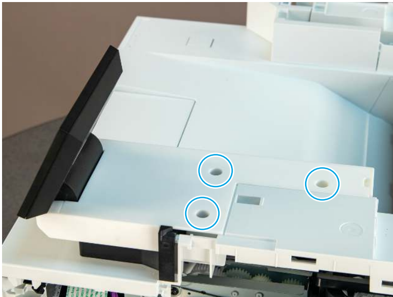
Figure 4-232 Remove three screws
