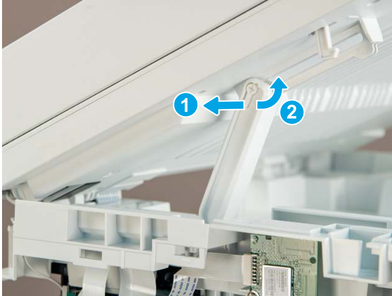
Figure 4-577 Remove the slider pin
