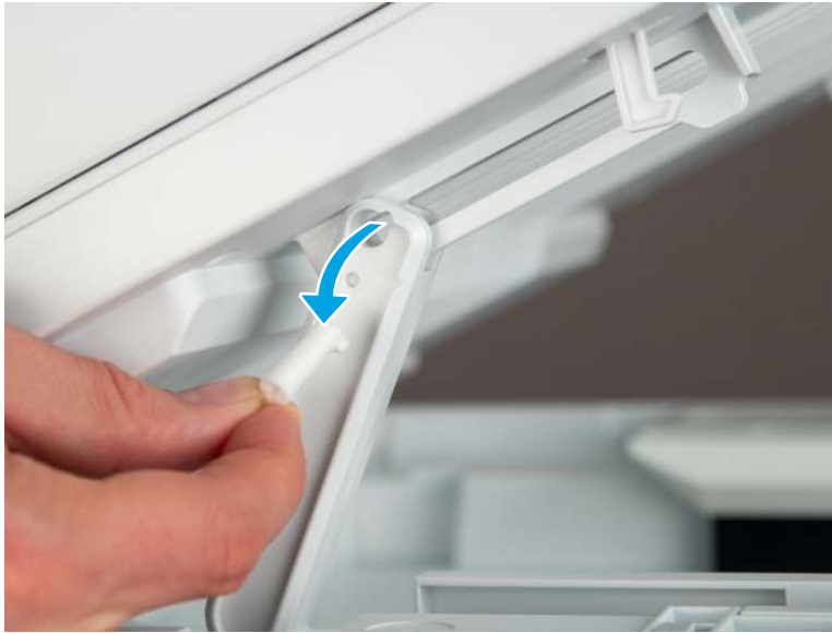
Figure 4-7 Remove the slider pin
