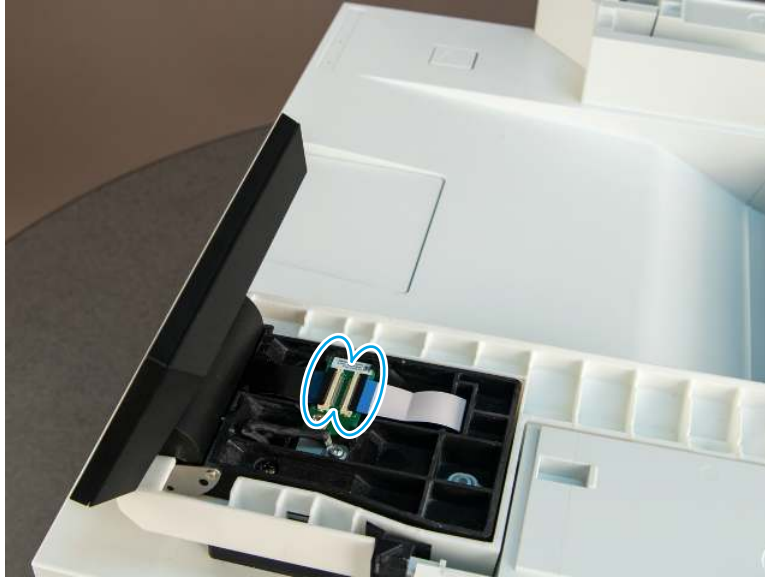
Figure 4-163 Disconnect two FFCs
