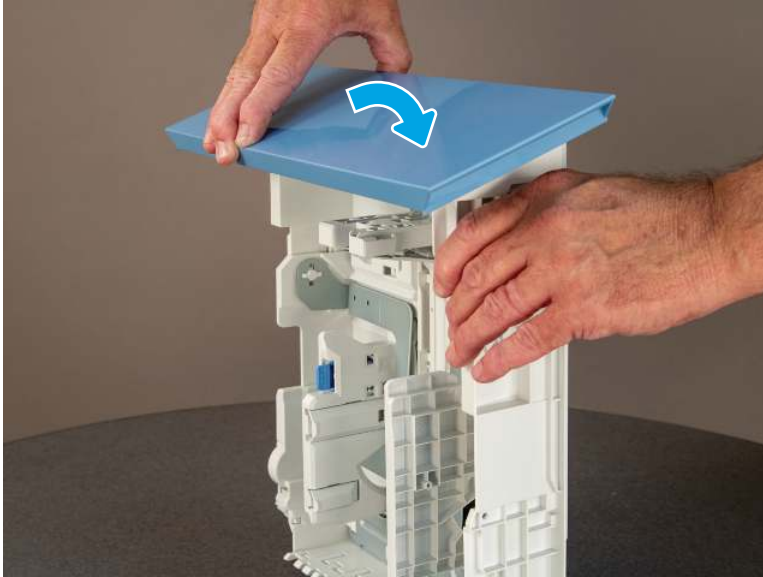
Figure 4-61 Install the cover
