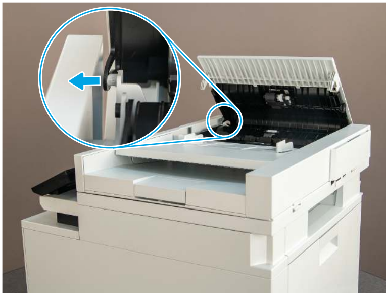
Figure 4-3 Release the clip
