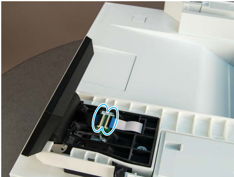
Figure 4-710 Disconnect two FFCs
