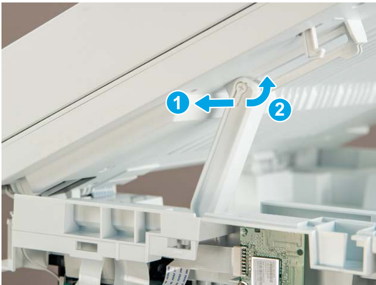
Figure 4-206 Remove the slider pin
