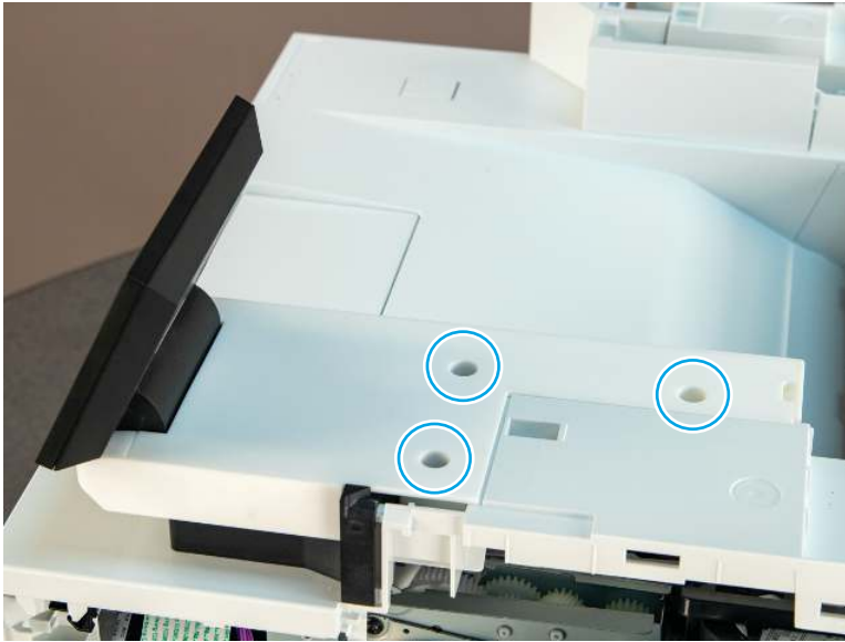
Figure 4-161 Remove three screws
