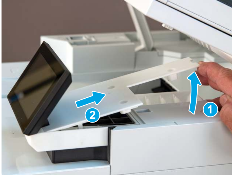
Figure 4-40 Remove the cover
