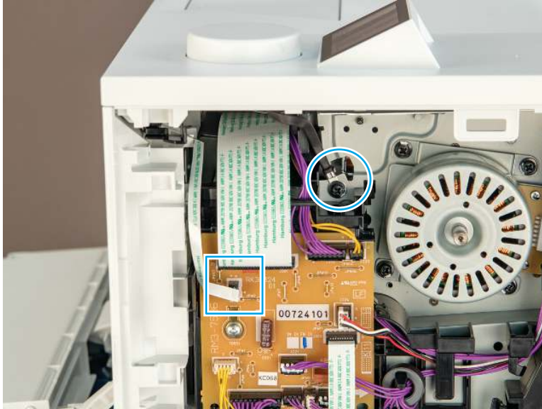
Figure 4-28 Disconnect one FFC and remove one screw
