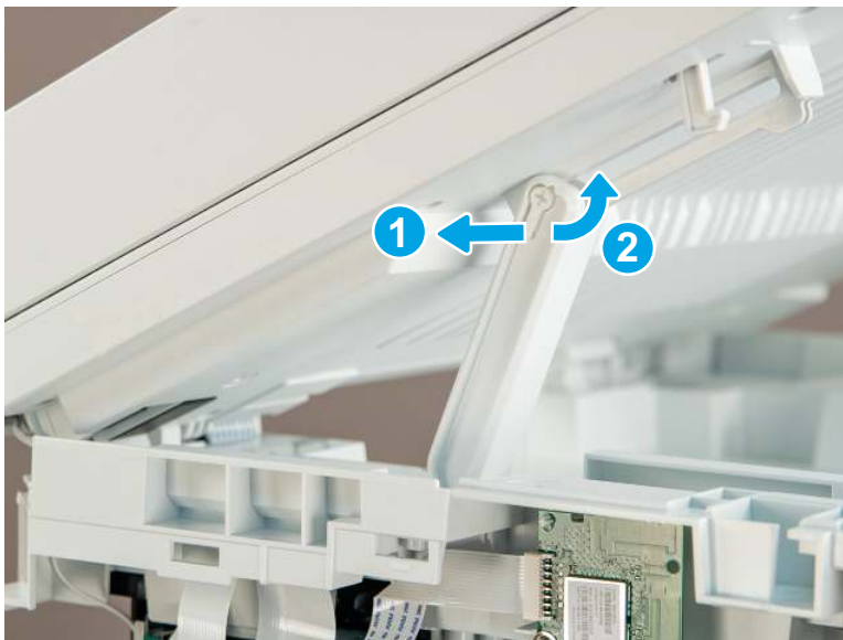
Figure 4-6 Release the slider pin
