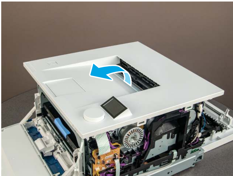
Figure 4-226 Remove the cover
