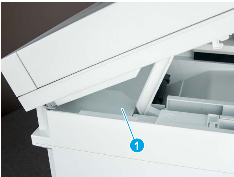
Figure 4-65 Remove the cover
