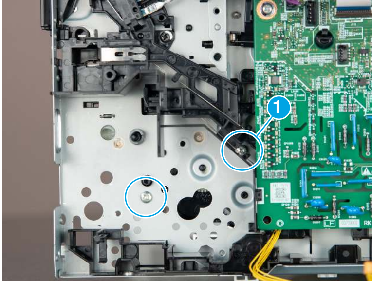
Figure 4-1135 Remove two screws
