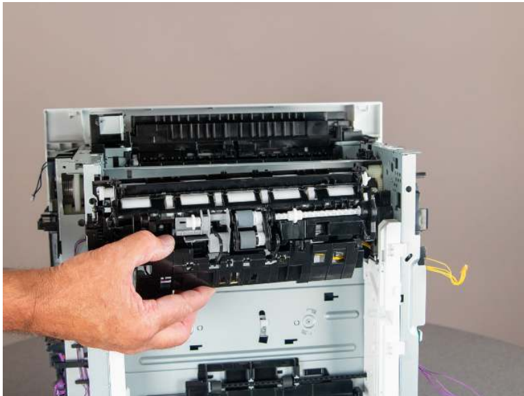
Figure 4-1134 Remove the feed upper guide assembly
