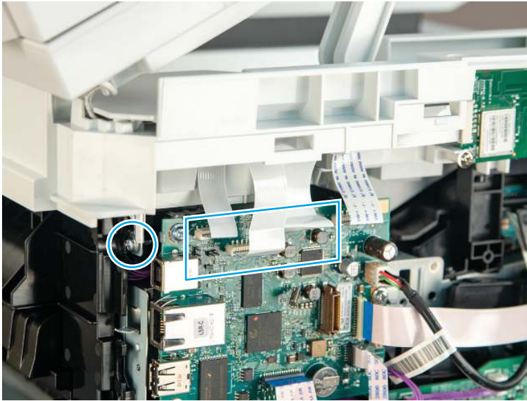
Figure 4-205 Disconnect FFCs and remove screw
