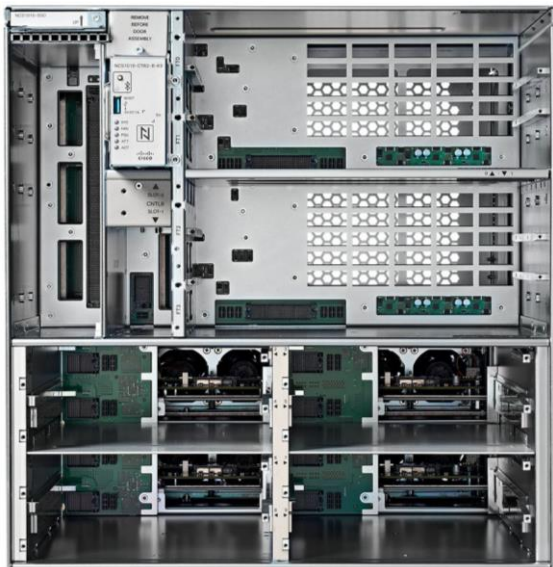
Figure 9. An empty NCS 1020 chassis
