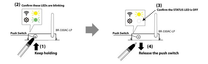
**6.** BR-330AC-LP will start to communicate with your wireless router. When the wireless configuration is successfully completed, the WLAN LED turns on and the STATUS LED turns on or blinks.
