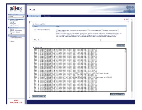
When the system log is saved, the event log and the other files are generated that will include the operating status.
