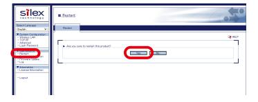
**3.** When the POWER LED and WLAN LED turn on, the restart is completed. After the restart, the BR-330AC-LP will start in a normal mode.
