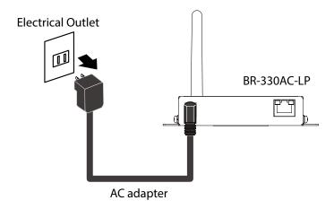
2. Plug the AC adapter back into the outlet.
