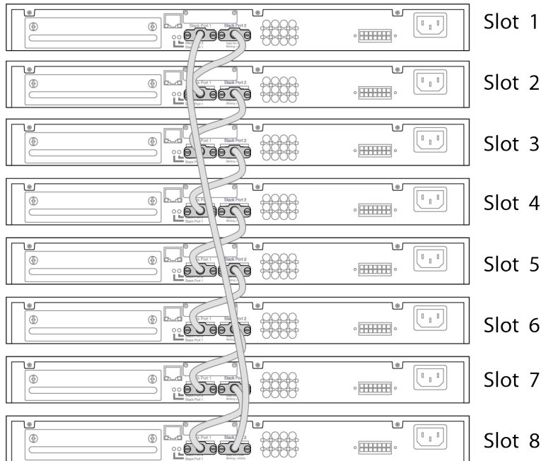
Figure 14: SummiStack Cable Connections Using Eight Switches with Integrated SummiStack Ports
