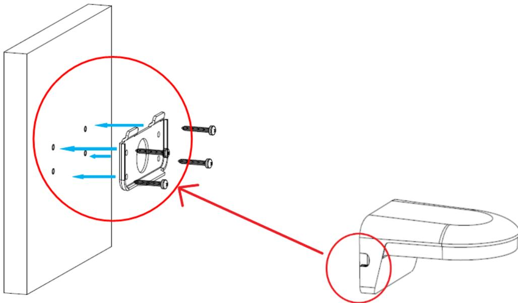
3. Fix the camera's collar onto UA-Mount215 with supplied screws.
