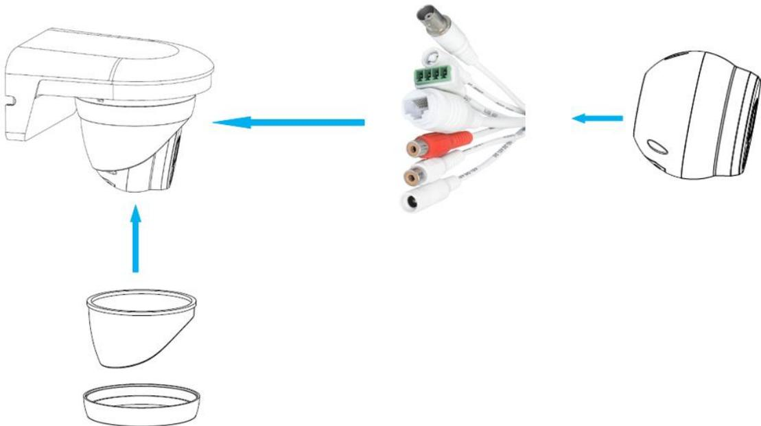
5. Connect the cables from the side hole of UA-Mount215 and tighten the bottom screw to complete the installation.
