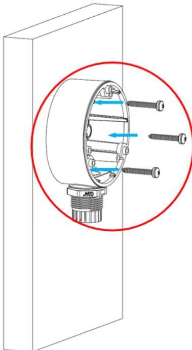
3. Thread the necessary cables from the bottom hole of UA-Mount505.
