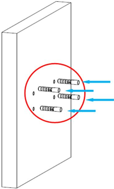
2. Secure the bottom plate of UA-Mount215 on the wall using the supplied screws.
