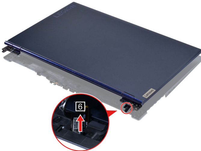
Figure 71. Take out the EDP cable and then remove the LCD module
