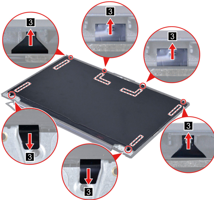
Figure 74. Remove the six pieces of removable tape with tweezers
