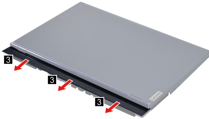
Figure 68. Remove the strip cover
