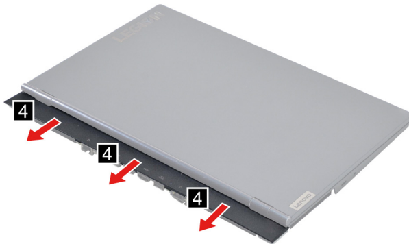
Figure 29. Remove the strip cover
