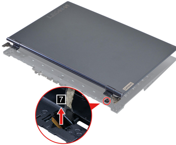
Figure 32. Take out the EDP cable and then remove the LCD module
