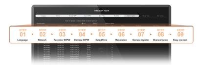
Wisenet A series NVRs walk users through the process of setting network, camera, and data and time settings using an easy and intuitive installation wizard.
