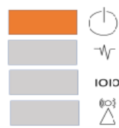
Figure: Power supply does not have redundancy
