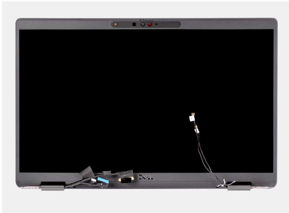
Figure 3. Display assembly with WWAN-antenna cables
