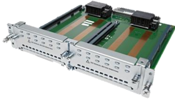
Figure 4. Cisco single-wide service module carrier card for 2x NIMs (C-SM-NIM-ADPT)
