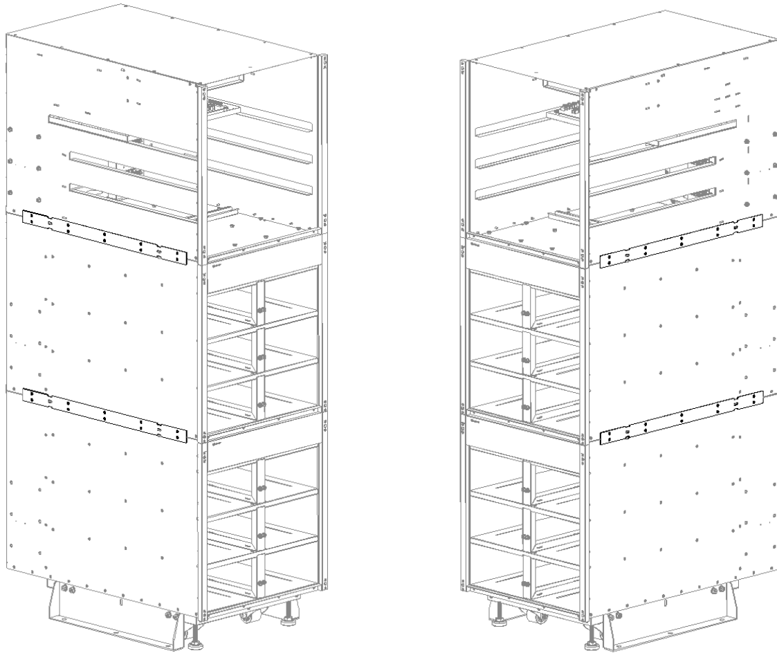
Fig 4-63: Secure the Side Straps Between UPS and Second Battery Cabinet (2)
